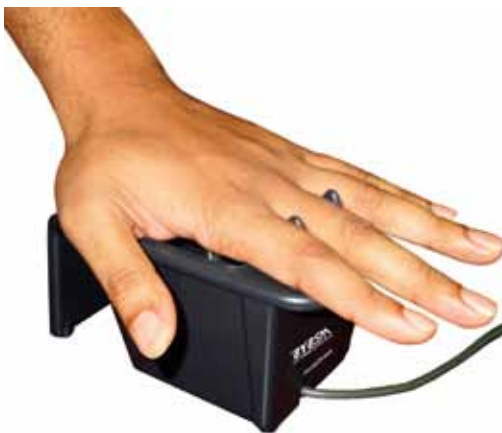
Figure 3 An example of a vein pattern recognition device. 2
